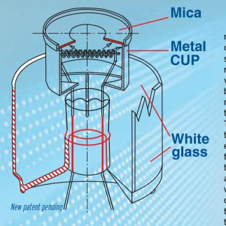
metal cover (the cup cathode). That may sound simple, but on closer review, it turns out to be a very clever design that brings far-reaching improvements compared with traditional lamp types. The sheath both optimizes the lamp's thermal efficiency and radically reduces the loss of emission material at the lamp ends. As a result, lamps can operate without blackening throughout their useful life. Customers will always feel that they are using a new lamp.
