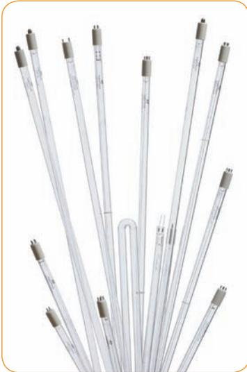
We offer our clients Very High (VH) germicidal lamps which generate energy at 185 nanometers (nm) in addition to the Low (L) 254 nm line. VH lamps are made with clear fused quartz and L lamps are made with a specially doped fused quartz that prohibits the emission of energy at 185 nm. VH lamps are used in a variety of
