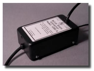
This unit measures approximately  $5.25^{\circ}$  L x  $3.0^{\circ}$  W x  $1.75^{\circ}$  H. It has two cords with plugs: one goes into the timer and one goes directly to 110Vac outlet. The 1200-CONTACTOR increases the power handling capabilities of any timer to 1200 Watts inductive load. Aristo light will work with all mechanical timers
