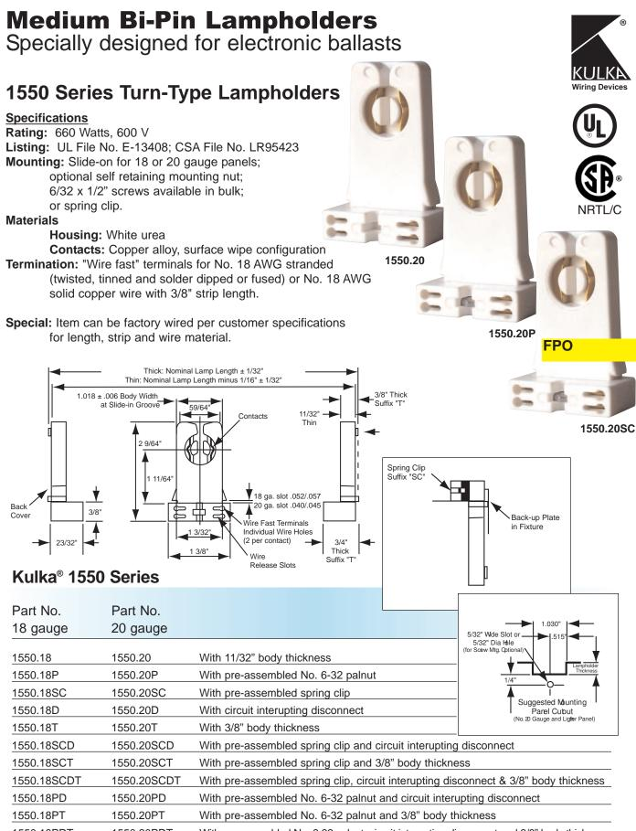
1550.18PDT 1550.20PDT With pre-assembled No. 6-32 palnut, circuit interupting disconnect and 3/8" body thickness
