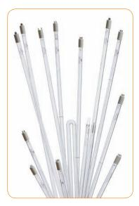
or envelope, of a germicidal lamp determines the wavelengths of ultraviolet (UV) emissions that react with the oxygen in the air to produce ozone. Ozone is an extremely active oxidizer. It destroys microorganisms on contact and also acts as a deodorizer. One of the primary advantages of ozone is that it can be carried by air into places that UV radiation cannot directly reach.
